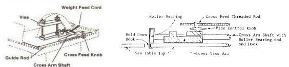
Weight feed action for slabbing utilizes a scale, cord, and weights fastened to vise. Deluxe power feed models with overrunning clutch and cut-off switch are available.
