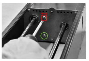
Adjust the belt tension by moving screw indicated above. Loosen the motor pivot screw marked in green first to allow for easy adjustment.
